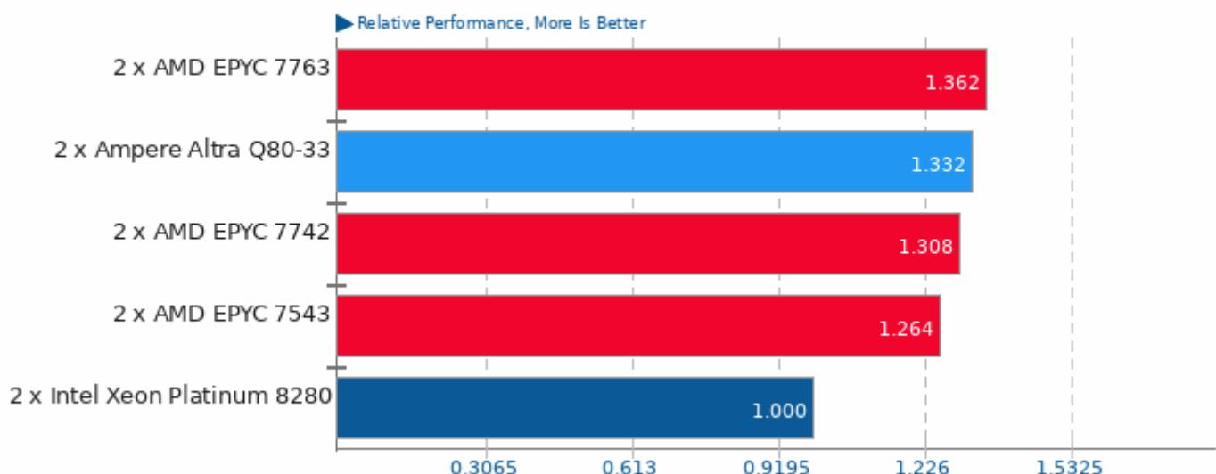
Geometric mean based upon tests: pts/rodinia, pts/build-llvm and pts/hpcg
